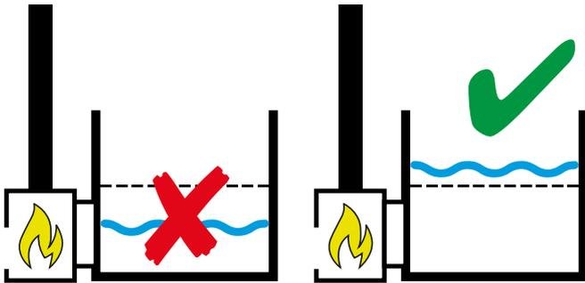
Before starting heating, fill the hot tub with water up to the minimum level, i.e. approximately 5 cm above the upper pipe of the heater.
